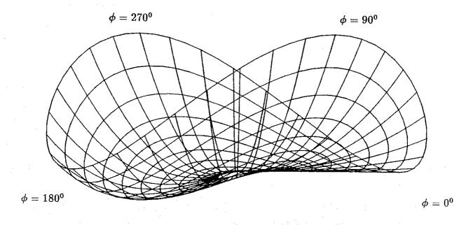
The second factor influencing total servo motion is the subtraction of an optimum baseline. The optimum baseline is selected for each  $\rho$  position. Its value is the mean of the height extremes as  $\phi$  progresses from  $0^{\circ}$  to  $360^{\circ}$ . The illustrations below, for the same outside segment, show two views of the servo tool motion with this optimum baseline subtracted.
