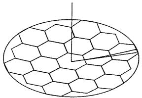
An example of this technology applied to a large segmented astronomical mirror is described below. In this example the parent surface is a paraboloid of revolution. The parent mirror functions at an optical speed of f/2.5, with a diameter of 80 inches and focal length of 200 inches. The mirror consist of 19 segments which are hexagonal as viewed along the optical axis. These segments are divided into 4 types: a center segment and three expanding rows of six segments each.
